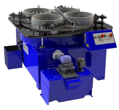
The Lapmaster Model 56 is equipped with a 1422mm diameter lap plate. This is manufactured from Grade 300 grey cast iron to ISO 185(2005). It consists of individual segments bolted to a support plate.
